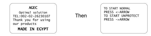
Now press left arrow **C** to run the charger normally with protection or press right arrow **C** to run the charger without protection for maintenance and change settings
