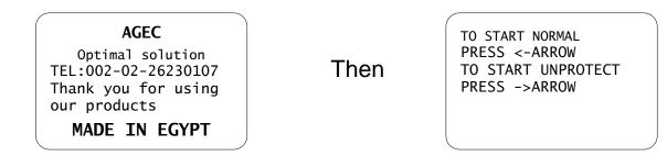
Now press left arrow to run the charger normally with protection or press right arrow to run the charger without protection for maintenance and change settings
